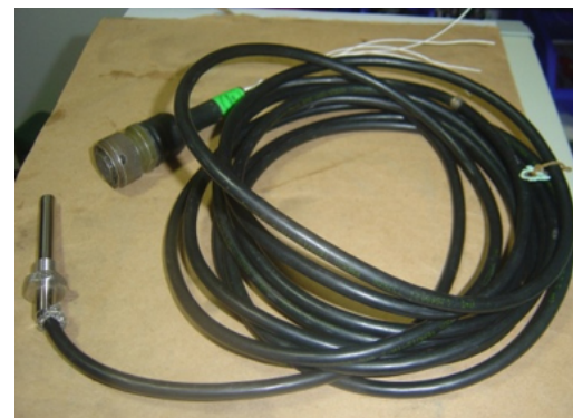
TEMPERATURE SENSOR OIL CIRCUIT TRANSFORMER –NS1010.08
